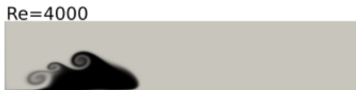
Figure 5. Snapshot of the concentration field (black c^* = 1 , white c^* = 0 ) at time t^* = 4.6 .
