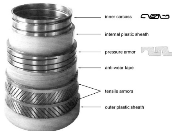
Figure 1. Typical Flexible Pipe [2]
