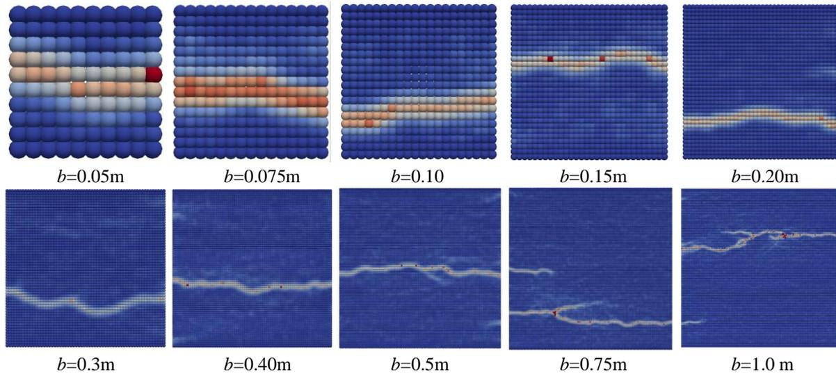
Figure 6. Damage distribution and rupture configuration of specimens of various sizes
