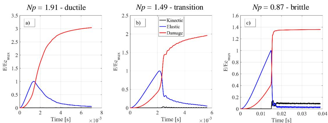
Figure 7. Evolution of the energies involved during the fracture process for the different classified behaviors
