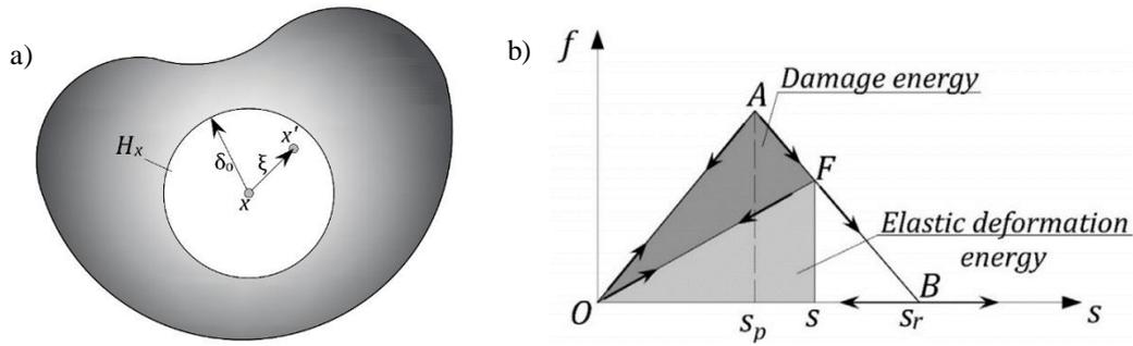
Figure 2. a) PD parameters [7], b) bilinear law and its relation with the involved energies in the loading process [10].
