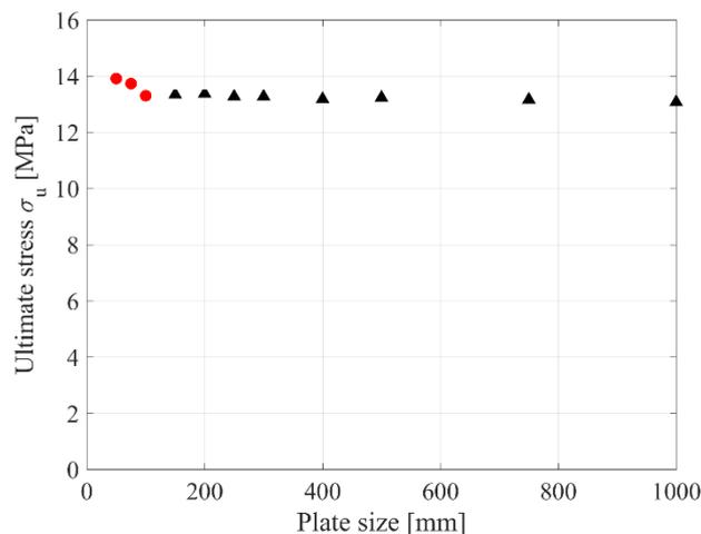
Figure 5. Ultimate global stress versus place size
