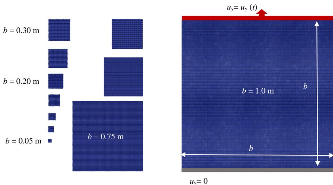
Figure 3. Relative plate dimensions and boundary conditions applied
