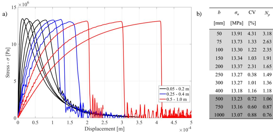
Figure 4. a) Displacement versus stress and b) Mean values of peak stress, coefficient of variation (CV) and stress brittleness number ( $N_p$ )
