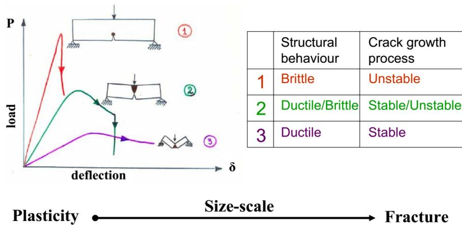
Figure 1. Illustration of the scale effect on beams of different sizes and their global behavior (adapted from [8])
