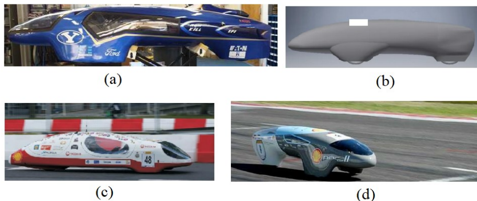
Figure 4. Models used as inspiration for the Models 2 and 3. (a) BYU Supermileage ( CD = 0.107 ) by Such [8]; (b) Si Pitung G4 ( CD = 0.13 ) by Sirojuddin et al. [9]; (c) Eco-Arrow ( CD = 0.096 ) by Such [8]; Pac-Car II ( CD = 0.075 ) by Such [8].
