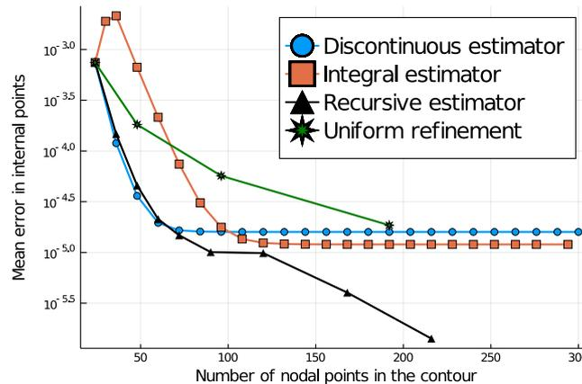
Figure 8. Variation of the average error in the internal points with the increase of the nodal points in the contour for quadratic elements.
