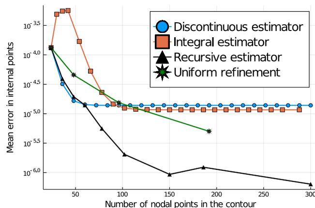
Figure 6. Variation of the average error in the internal points with the increase of the nodal points in the contour for quadratic elements.
