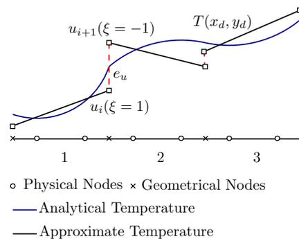
Figure 1. Schematic drawing of the discontinuous error estimator.
