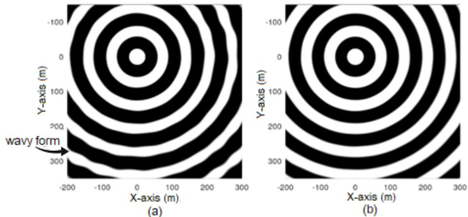
Figure 3. The 30-Hz time-domain solution of the P-wave field in a homogeneous medium for the instant of time  $t = 0.8325$  s. (a) for ABC-1D, and (b) for ABC-2D.
