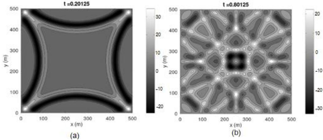
Figure 2. The 30 Hz time-domain solution of the P-wave amplitudes in a homogeneous medium with full reflection boundary condition.
