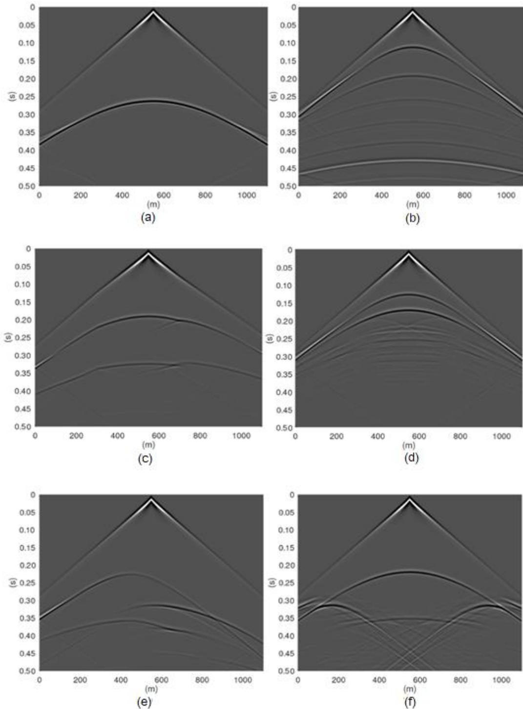
Figure 4. Synthetic seismograms referring to the six seismic models. (a)  $M_I$ , (b)  $M_{II}$ , (c)  $M_{III}$ , (d)  $M_{IV}$ , (e)  $M_V$ , and (f)  $M_{VI}$
