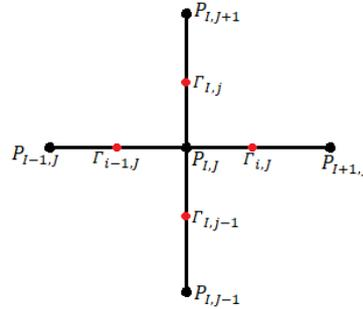
Figure 1. Schematic grid representation of unknown Pressure (the  $P$ -points) and know information at middle grid points (the  $\Gamma$ -points).
