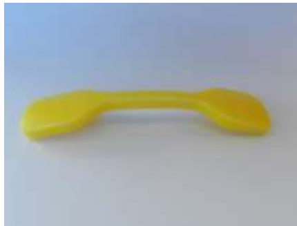
Figure 2. HDPE specimen employed for creep-recovery test
