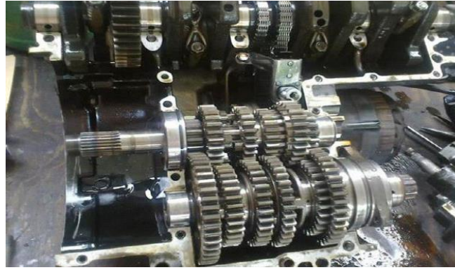
Figure 1. Honda CBX 750F motorcycle gearbox. Source: Design by the author
