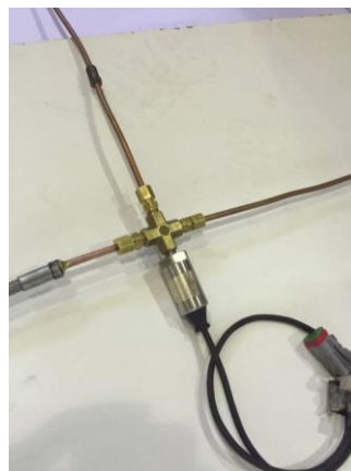
Figure 5 – Pressure sensor – front line tubing.
