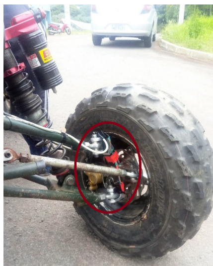
Figure 2. Instrumented front stub axle (Author)
