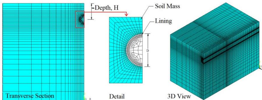
Figure 1 - Three-dimensional model for tunneling.
