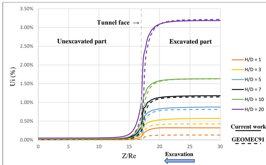
Figure 2 - Convergence curves according to  $H/D$ : comparison between Ansys (current paper) and GEOMECC91 (Bernaud and Rousset's [21]) results.
