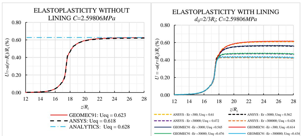
Figure 5. Examples of verification of the tunnel models in elastoplasticity without/with elastic lining
