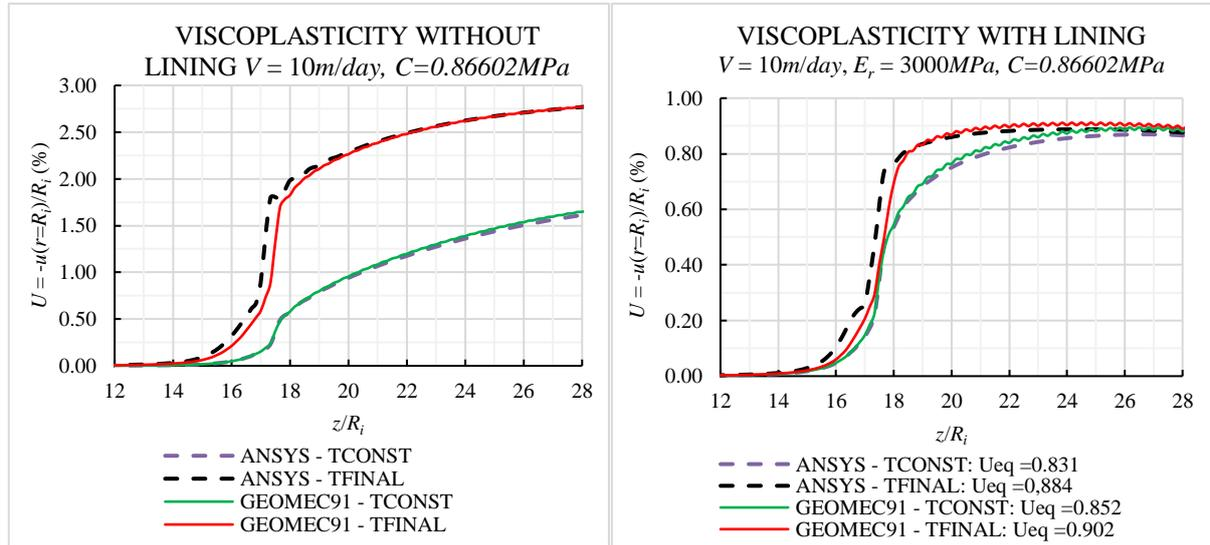
Figure 6. Examples of verification of the tunnel models in viscoplasticity without/with elastic lining
