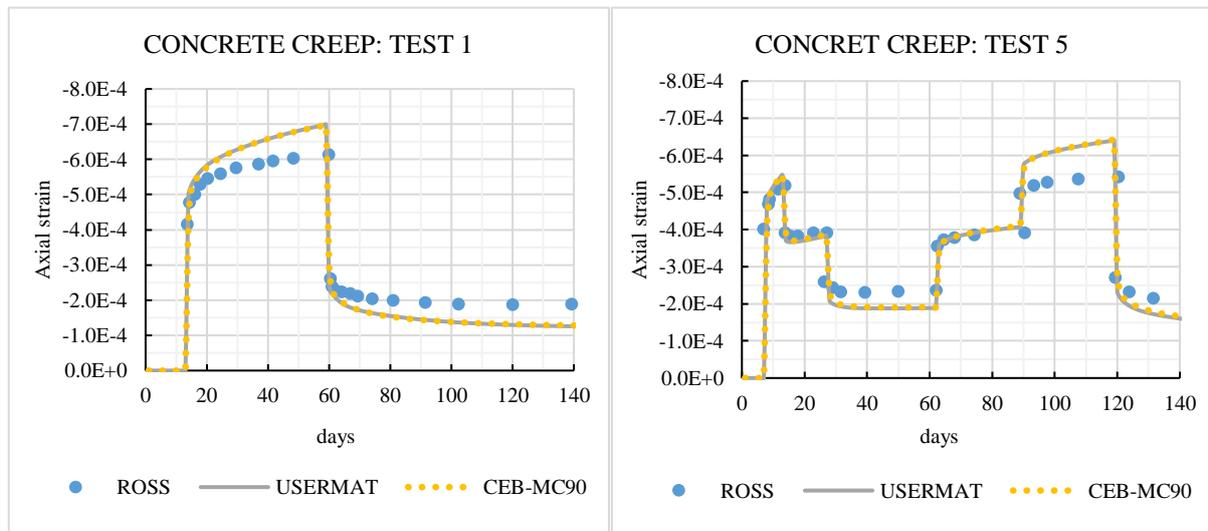
Figure 4. Examples of verification of the concrete constitutive model
