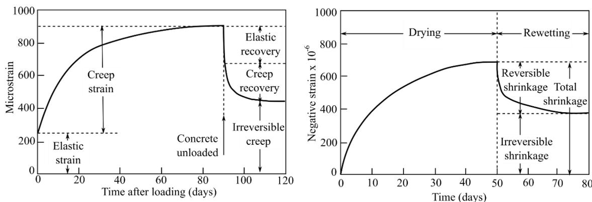
Figure 2. (a) typical shrinkage curve of concrete, (b) typical creep curve of concrete (MINDESS et al. [14])
