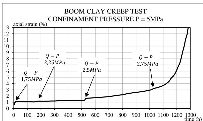
Figure 1. Boom clay creep test (Rousset [12])
