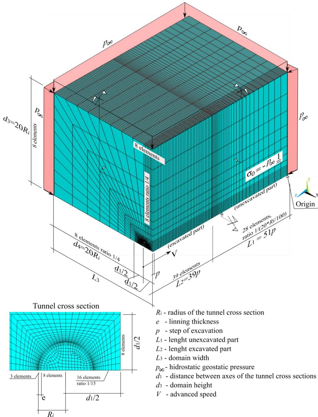
Figure 3. Mesh, geometric parameters and boundary conditions for twin tunnels
