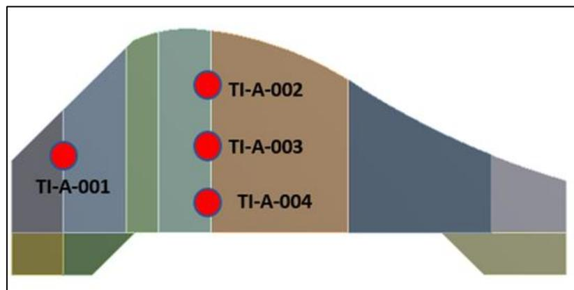
Figure 13. Location of the internal thermometers of block A-7. (Source: the author,2020)
