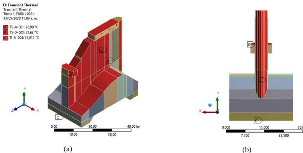
Figure 11. Thermal boundary conditions (a) Isometric View, (b) Rear View. (Source: the author,2020)
