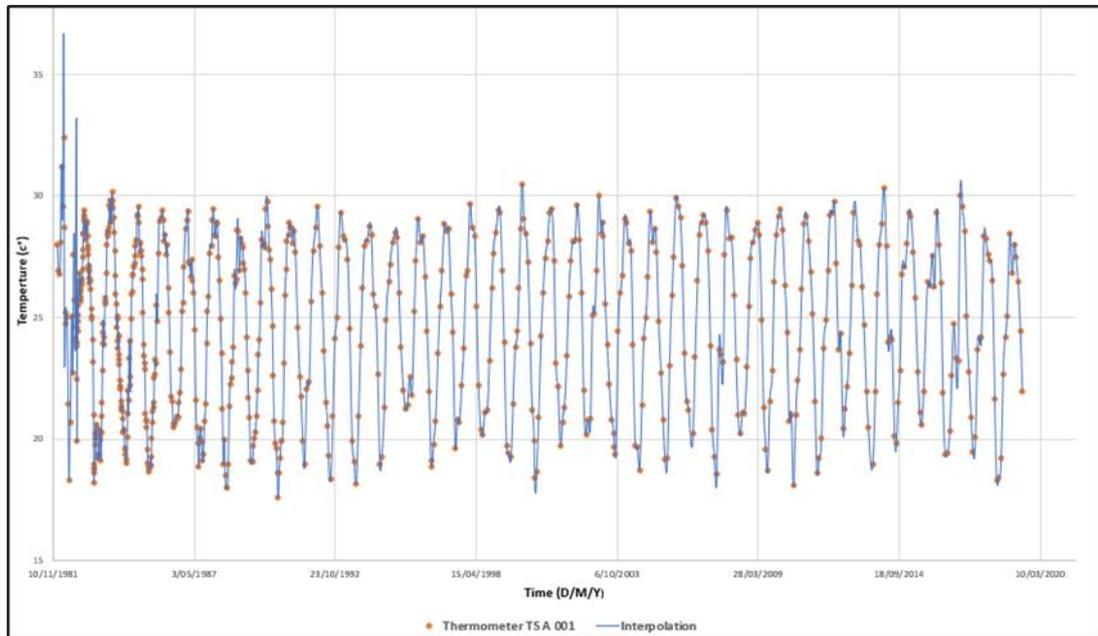
Figure 8. Interpolation of the thermal data of the TS-A-001 thermometer (Block A-7). (Source: the author,2020)
