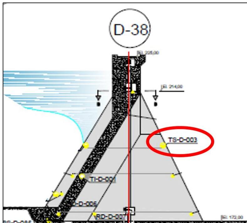
Figure 7. Block D-38 Instruments (Source: SAT [8])
