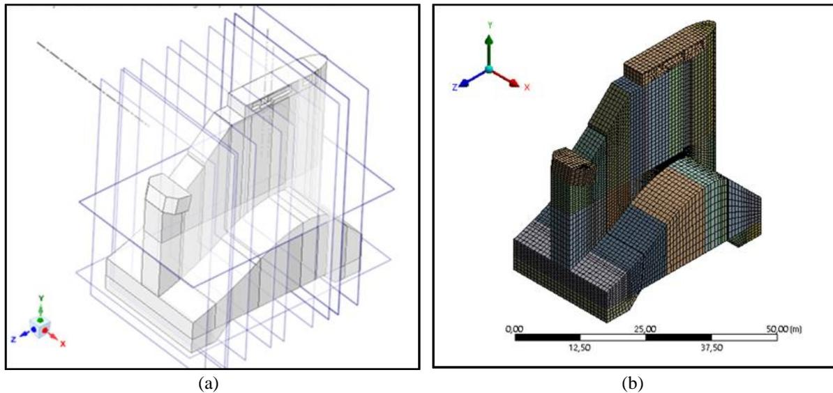
Figure 5. (a) Geometric model division, (b) Mesh. (Source: the author,2020)
