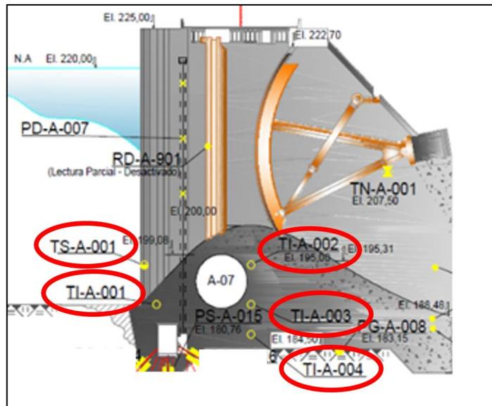
Figure 6. Block A-7 spillway instruments. (Source: SAT [8])
