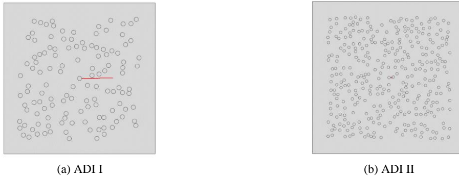
Figure 6. Crack propagation for cases with nodules randomly positioned
