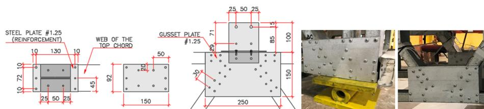
Figure 3. (a) The TWP shear connector; (b) detail of the CFS truss at the support; (c) typical joint of the truss with gusset plate and self-drilling screws (Leal [6]).
