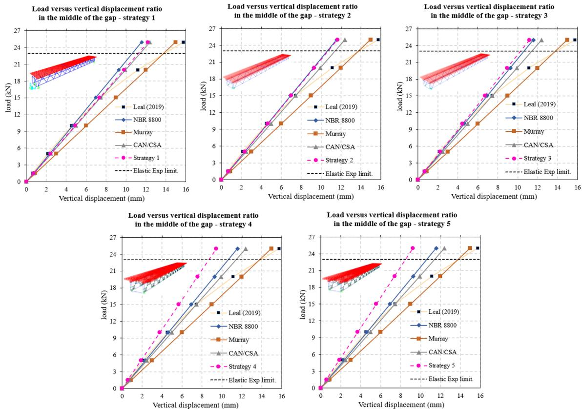
Figure 7. Applied force vs. mid span vertical displacement according with FEM model strategies (a) 1; (b) 2; (c) 3; (d) 4 and (e) 5; and the computed results of the analytical design rules from the Brazilian code ABNT NBR 8800, Murray (1997) and the Canadian code CAN/CSA.
