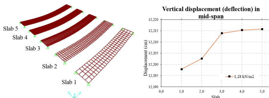
Figure 4. (a) The 5 models of the slab discretization; (b) the convergence results of the vertical displacement at the center of the slab.
