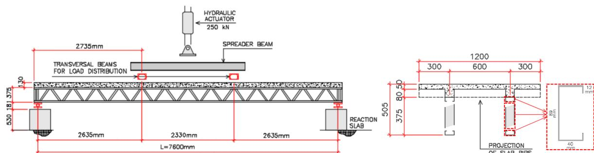
Figure 2. (a) Experimental set up of the four points bending test; (b) cross section of the floor system, dimensions in mm (Leal [6]).
