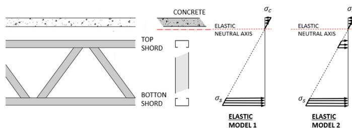
Figure 8. Analytical models for the computation of the strength capacity of the composite trussed beam system (Leal [6]).
