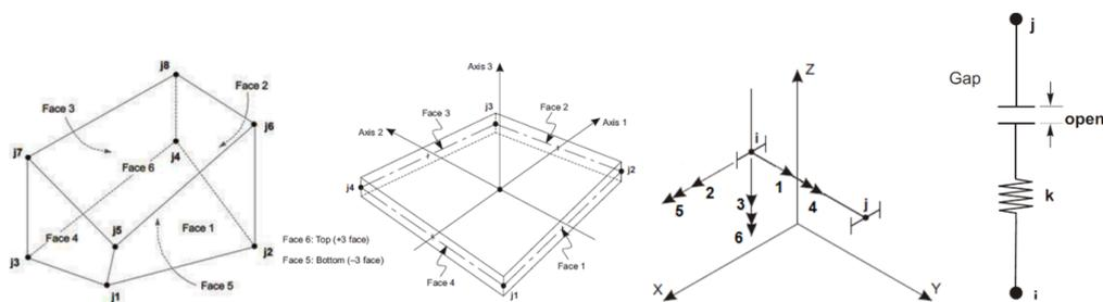
Figure 5. Applied finite elements: (a) solid; (b) shell; (c) frame and (d) gap (SAP2000 [8]).
