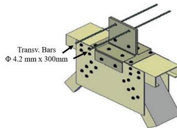
Figure 1. The TWP Thin-Walled Perfobond connected to the lipped channel CFS of the upper chord of the truss (Leal [6]).
