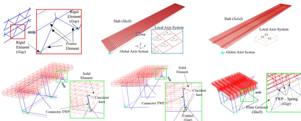
Figure 6. Illustration of the adopted FEM model strategies: (a) eccentricity at the joints of the truss; (b) shell slab; (c) slab with solid elements; (d) strategy 2; (e) strategies 3 and 4; (f) strategy 5.
