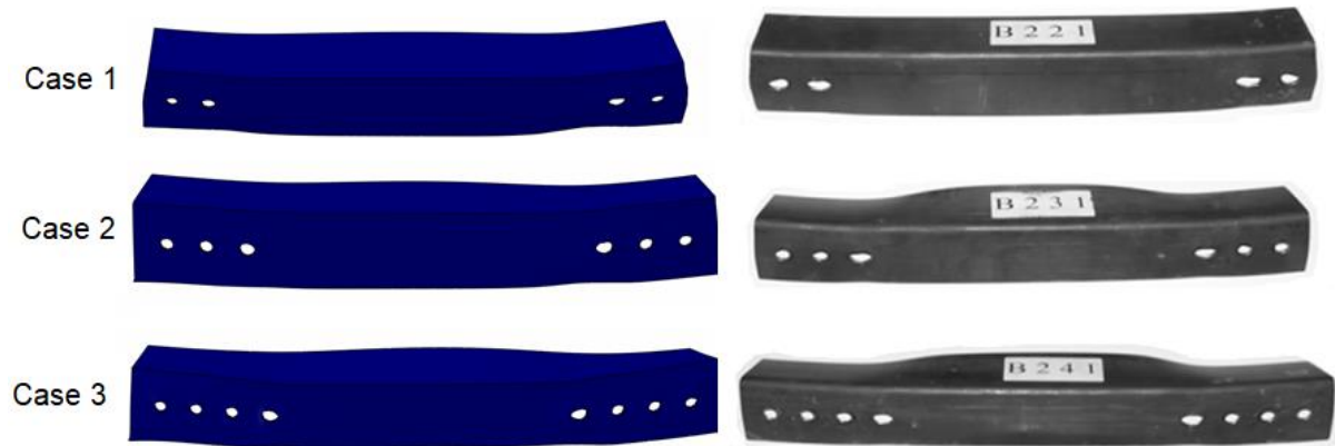
Figure 8 - Numerical and experimental deformation of the B221, B231 and B241 angle at the moment of ultimate load.
