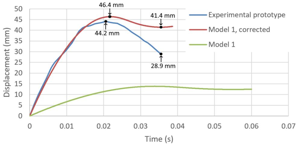
Figure 7. Impactor block displacement curve for Model 1, Experimental prototype, and corrected Model 1
