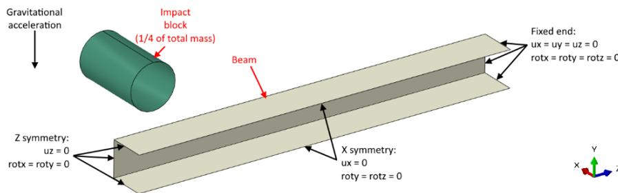
Figure 2. Boundary conditions applied to the beam
