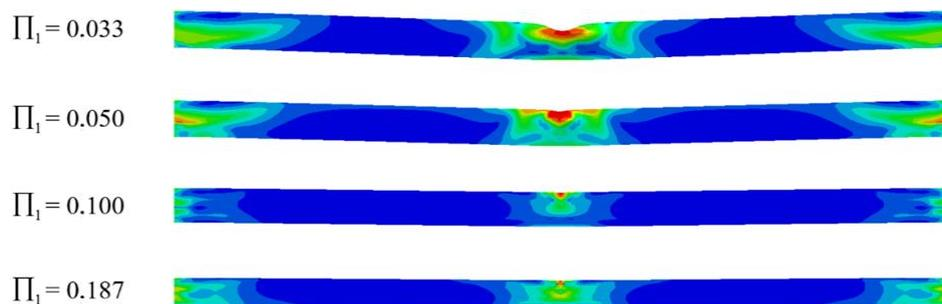
Figure 4. Permanent deformation profile of the beam for different values of  $\Pi_1$
