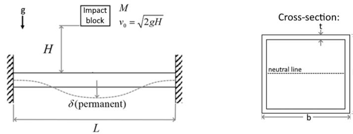
Figure 1. Schematic figure of the beam drop test problem
