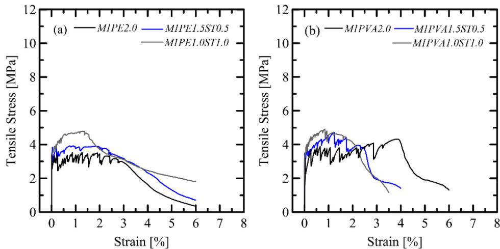
Figure 3. Representative stress-strain curves obtained for the following composites: (a) M1PE2.0 and hybrid systems and (b) M1PVA2.0 and hybrid systems.
