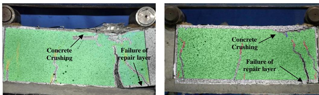
Figure 6. Failure modes of beam specimens: (a) repaired with M1PVA2.0 and (b) repaired with M1PE2.0.
