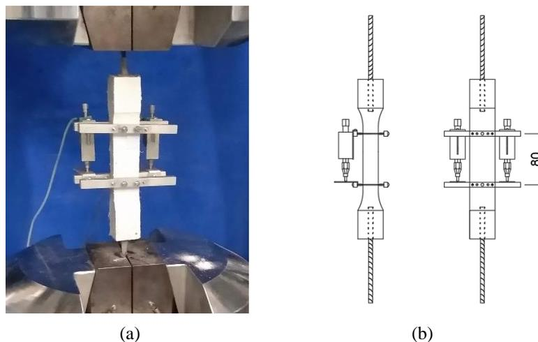
Figure 1. Direct tension test: (a) test setup and (b) details of the setup. Dimensions in mm.
