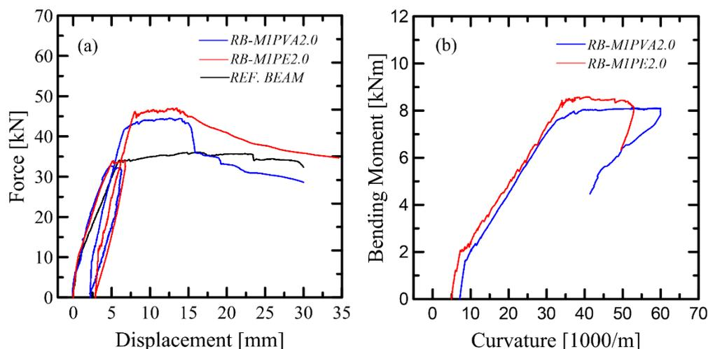
Figure 5. Results from structural tests: (a) load-displacement and (b) bending moment-curvature for the second loading.
