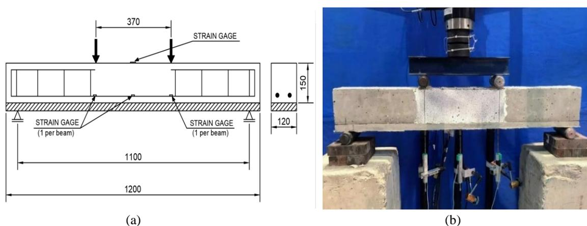
Figure 2. Structural test: (a) scheme of the test and (b) complete test setup (All dimensions in mm).
