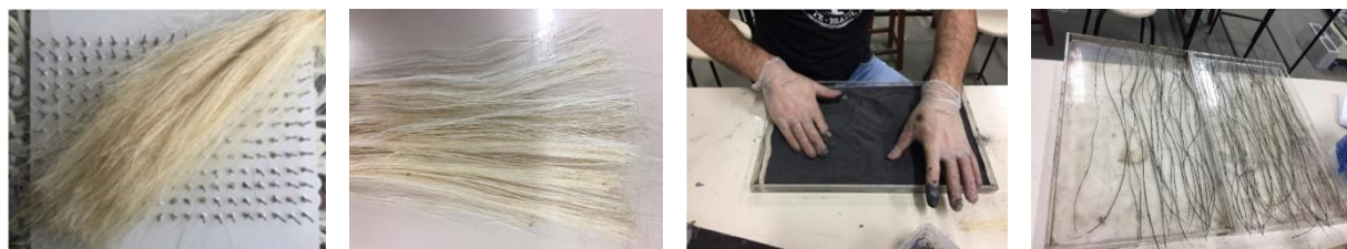
Figure 1. Surface treatment applied to the sisal fibers: (a) Untangling process, (b) fibers "in natura", (c) adhesion of ferromagnetic residue to fibers and (d) treated fibers before cutting.
