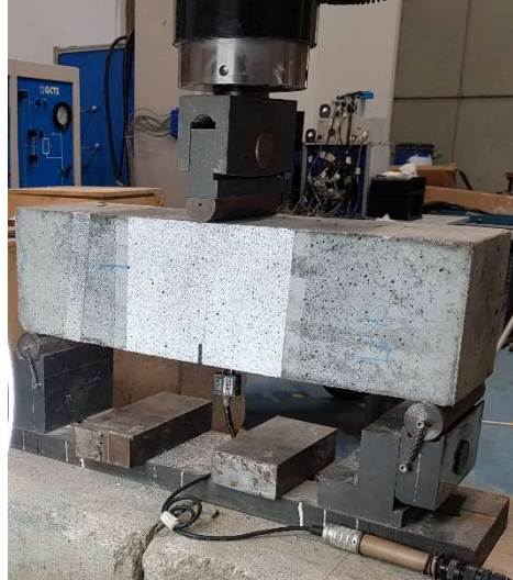
Figure 1. Three-point bending test setup
