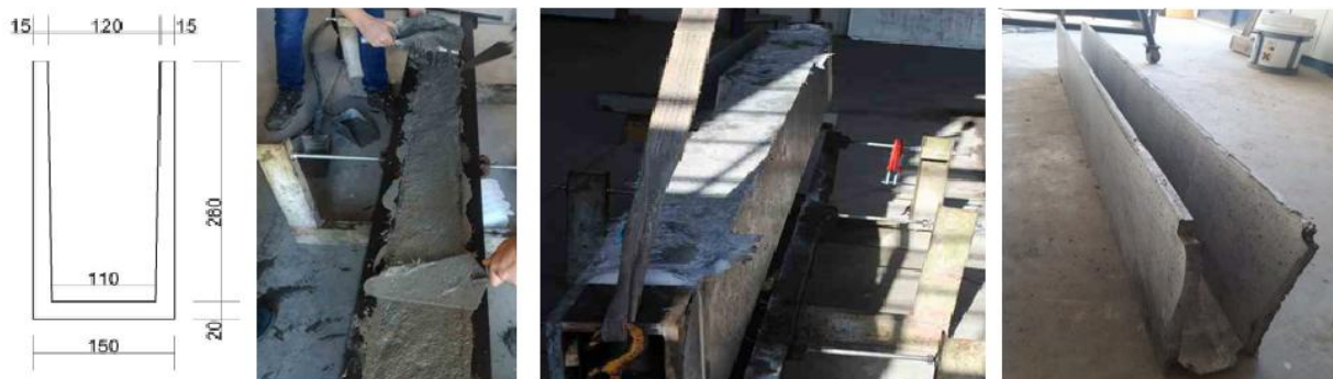
Figure 1. Production of the permanent forms
