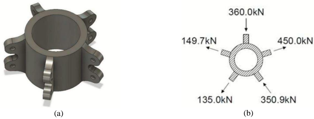
Figure 4 Cylindrical-shaped truss joint studied by Abdelwahab [4] (a) basic geometry; (b) load case
