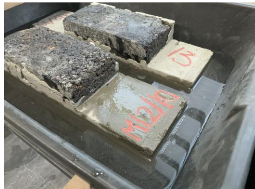
Figure 2: Curing process for the composite beams
