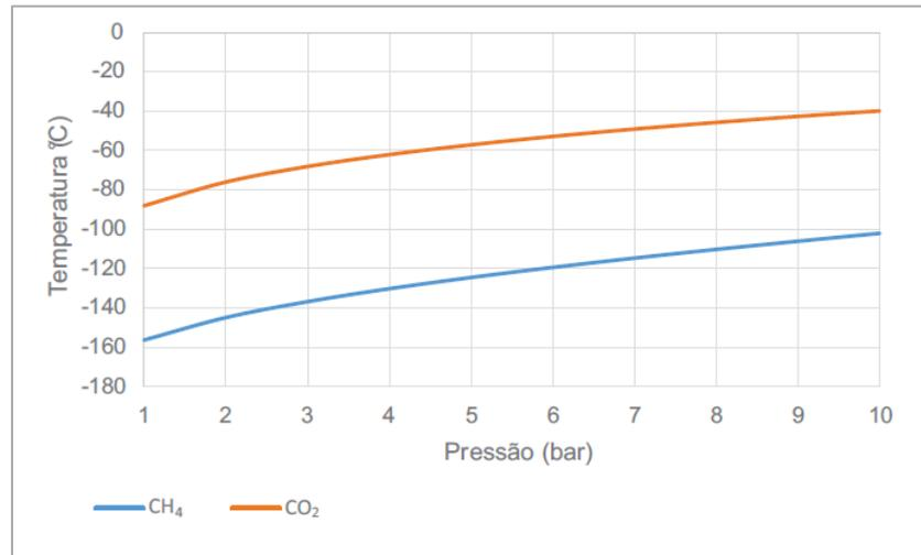
Figure 1. Boiling temperatures of methane and carbon dioxide indifferent pressures.
