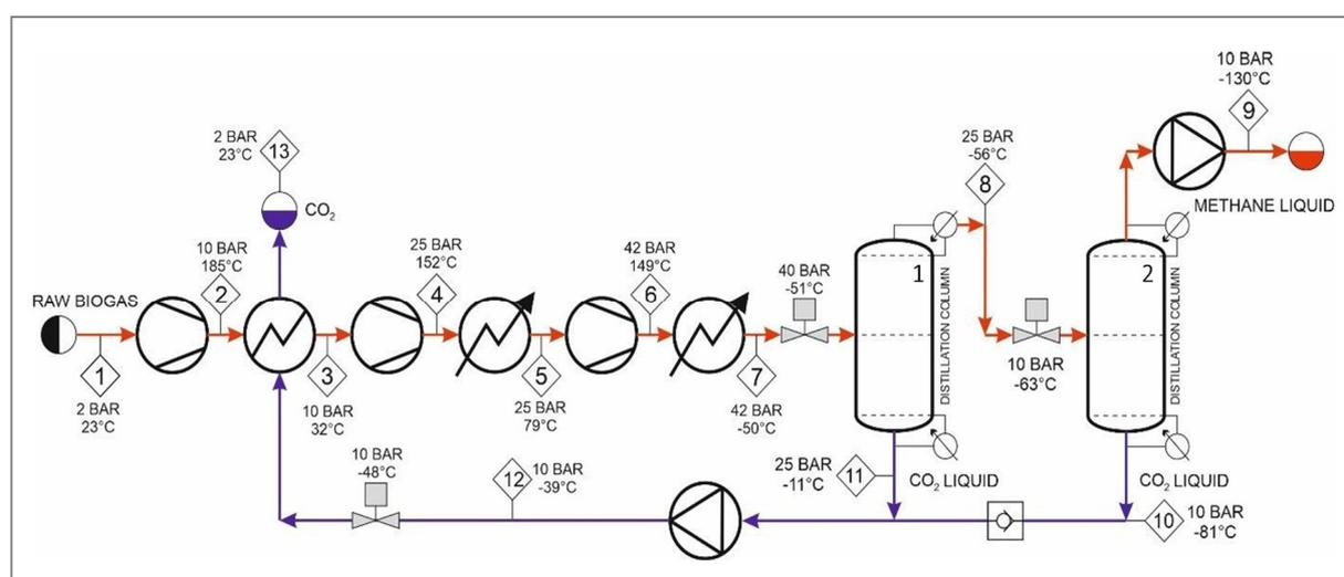
Figure 2. Upgrading cryogenic biogas
