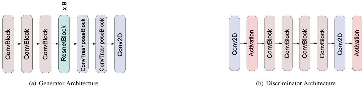
Figure 5. Schematic illustration of the architecture of the Generators (a) and Discriminators (b) of Cycle GAN.
