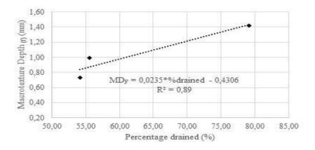
The line of equality equation was applied and then, calculated a model macrotexture depth  $(MD_M)$ . The model can predict the macrotexture classification in most cases. However, the model could not be satisfactory in open macrotextures. The results are presented in Table 1.
