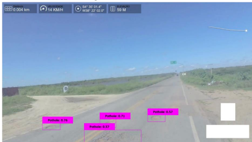
Figure 4. Defect detection by Yolov3 - 416x416 pixels model
