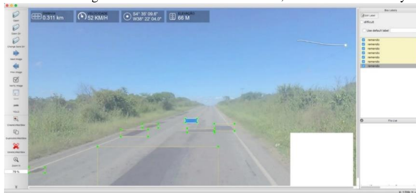
Figure 2 - Labeling of defects in the pavement
