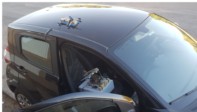
Figure 6. Attachment of the research device to a car for performing dynamic tests.
