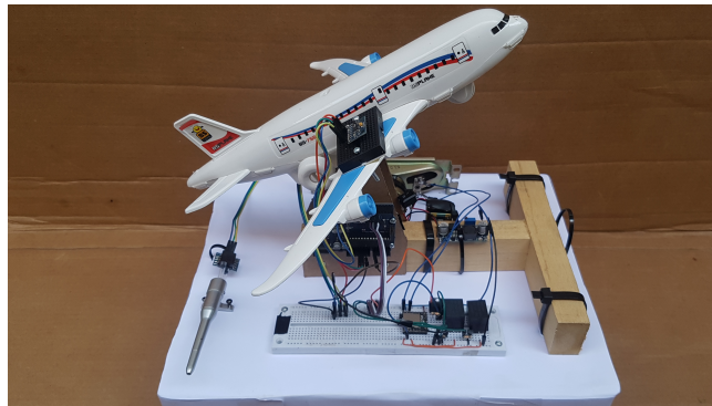
Figure 5. Didactic prototype developed for research to identify stall situations.
