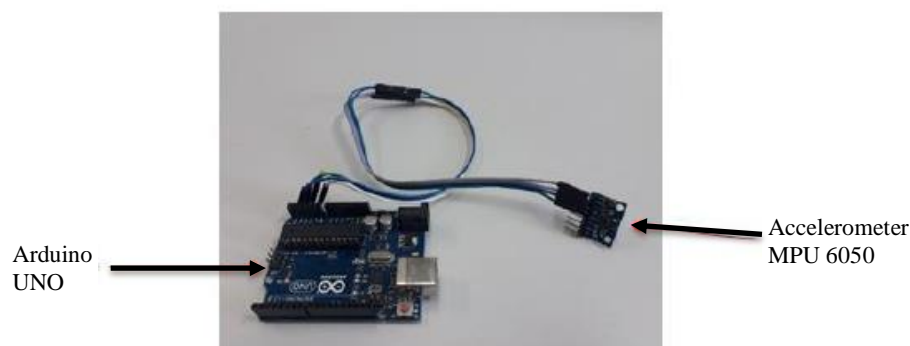
Figure 6 – Vibration Signal Acquisition System
