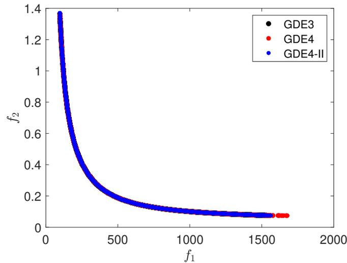
Figure 3. Pareto front obtained in the continuous structural multi-objective optimization design of the 72-bar trus.
