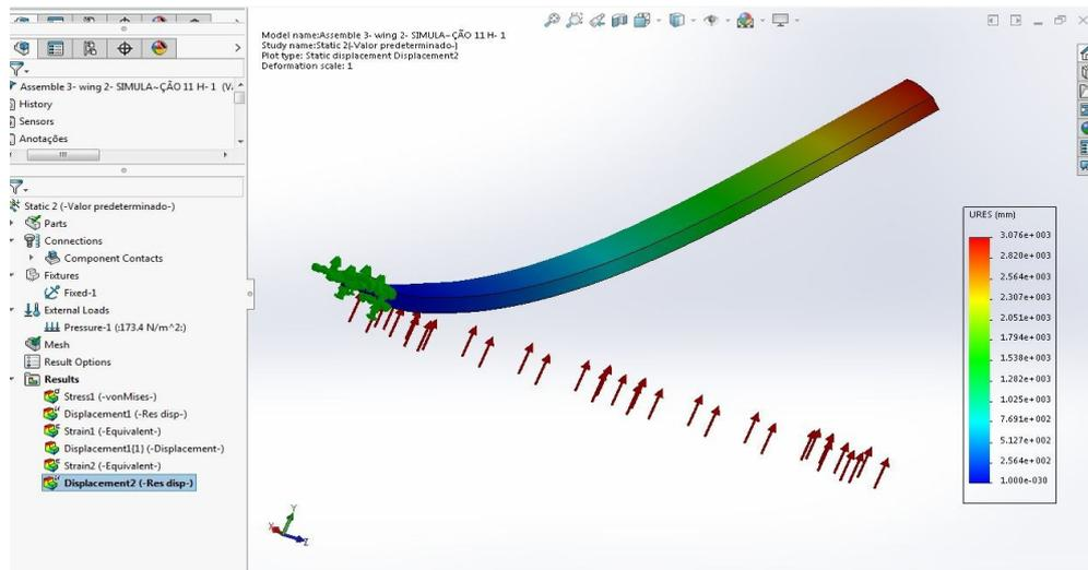
Figure 5. Main spar modeled with finite elements
