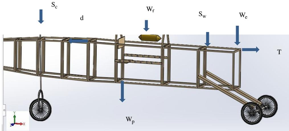
Figura 4. Simplified drawing of the fuselage of the airplane
