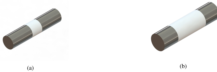
Figure 3. a) cell composed of 90% Steel and 10% Polyacetal b) cell composed of 50% Steel and 50% Polyacetal
