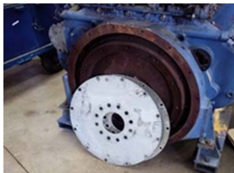
a) Flexible metal disk coupling (from Bretech Energia S.A. company)
