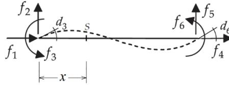
Figure 4. Nodal forces acting on pure deformational configuration
