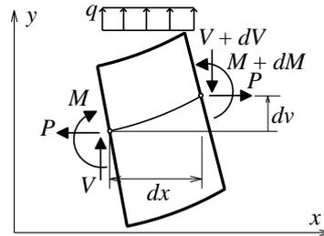
Figure 1. Equilibrium of the infinitesimal element
