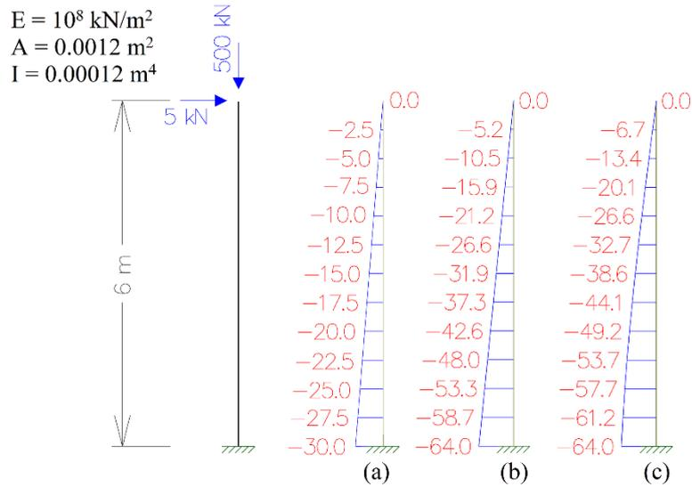
Figure 5. Example 1: (a) 1<sup>st</sup> order analysis; (b) 2<sup>nd</sup> order without P-δ; (c) 2<sup>nd</sup> order with P- δ
