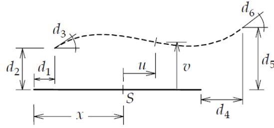
Figure 3. Deformed configuration of a frame element
