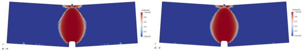
Figure 7. Crack pattern for damage model with Nonlocal integral: mesh 1 (top-left), mesh 2 (top-right), mesh 3 (bottom-left) and mesh 4 (bottom-right)
