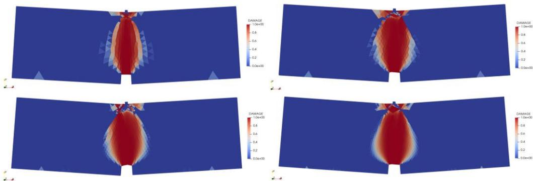
Figure 5. Crack pattern for damage model with Crack band: mesh 1 (top-left), mesh 2 (top-right), mesh 3 (bottom-left) and mesh 4 (bottom-right)
