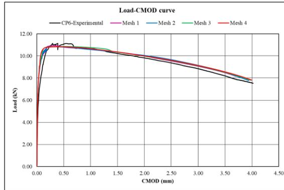
Figure 8. Load-CMOD curve for damage model with Nonlocal integral
