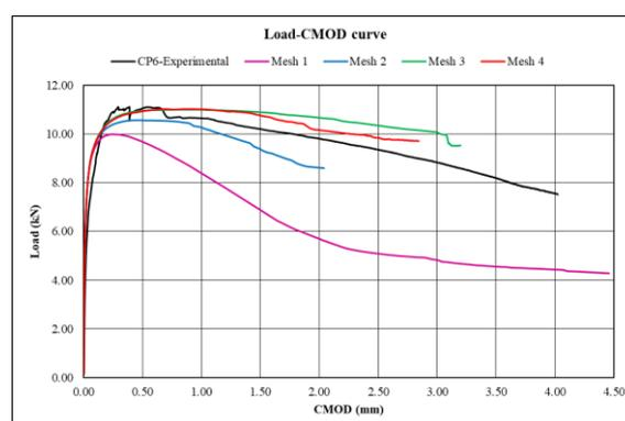
Figure 3. Load-CMOD curve for Smearred crack model with Crack band technique
