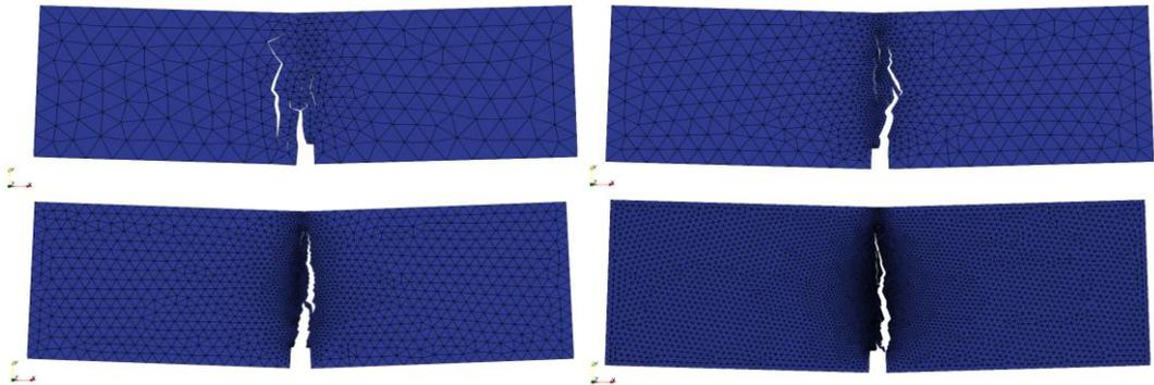
Figure 9. Crack pattern for Interface elements with Cohesive Zone model: mesh 1 (top-left), mesh 2 (top-right), mesh 3 (bottom-left) and mesh 4 (bottom-right)
