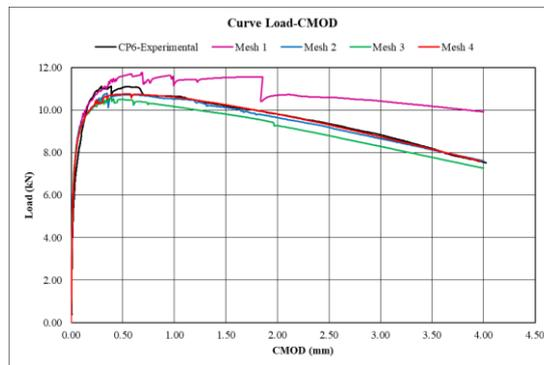
Figure 10. Load-CMOD curve for damage model with Interface elements with Cohesive Zone model
