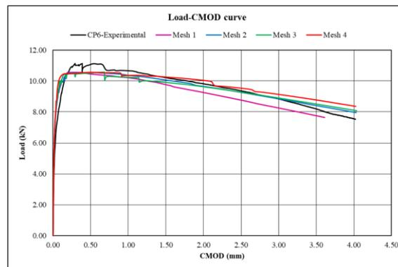
Figure 6. Load-CMOD curve for damage model with Crack band technique
