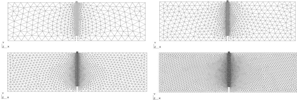
Figure 4. Mesh 1 (top-left), mesh 2 (top-right), mesh 3 (bottom-left) and mesh 4 (bottom-right)
