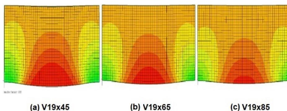
Figure 3. Stress distribution considering the column cross section as support
