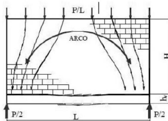
Figure 1. Redistribution of stresses in case of debonding in the center part of the span (Barbosa [5])
