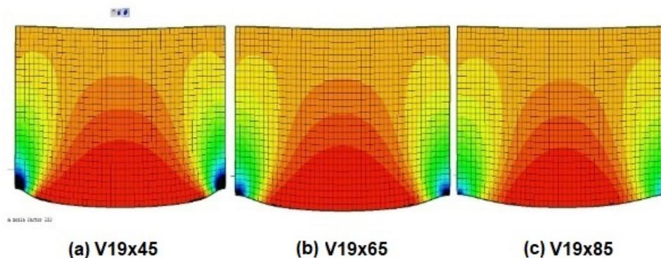
Figure 2. Stress distribution in the Wall for the cases involving the 4,6m beam
