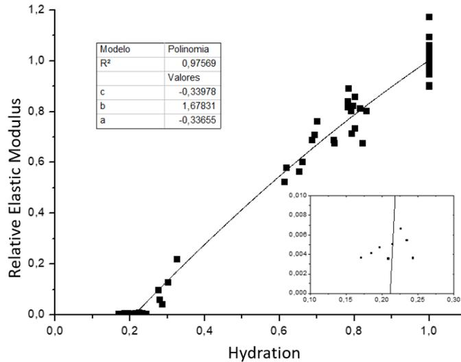
Figure 2. Relation between degree of hydration and relative elastic modulus
