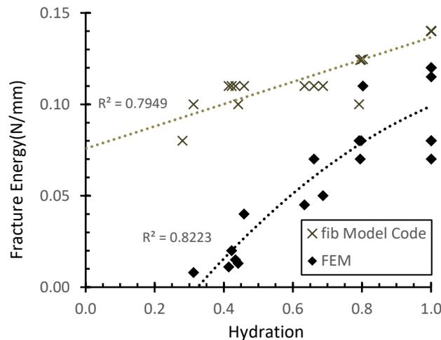
Figure 6 - Evolution curve for the fracture energy of the concrete according to the hydration degree. Comparison between FEM and Model Code results
