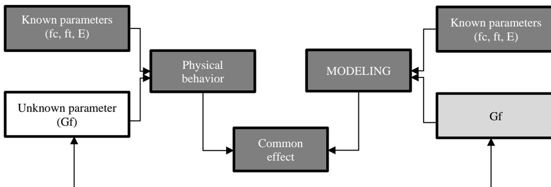
Figure 3 - Inverse analysis procedure
