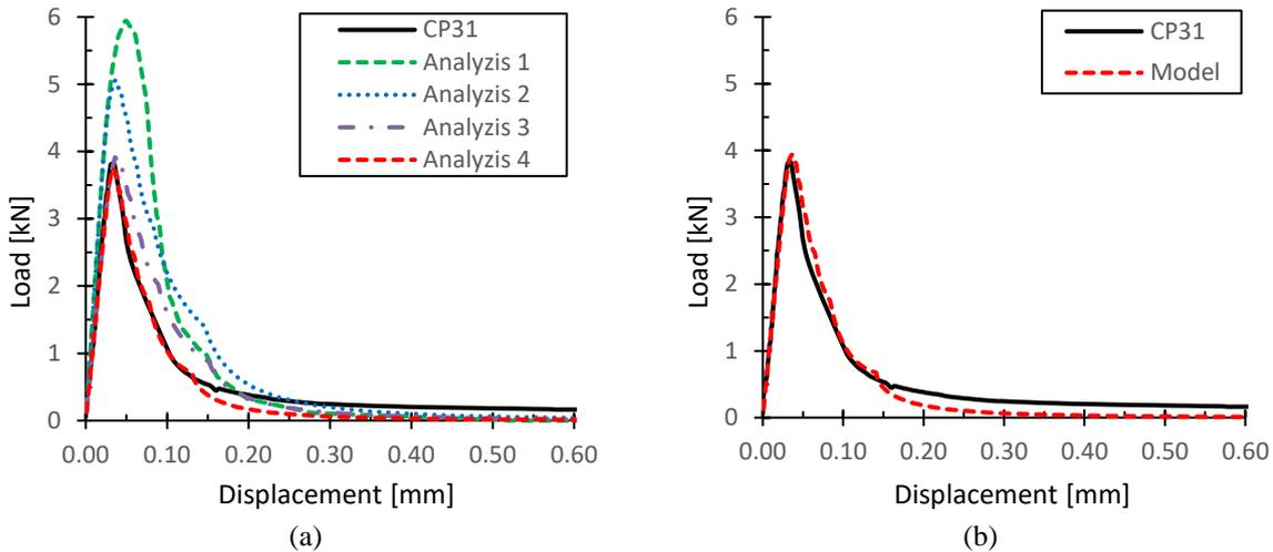
Figure 5 – Example of procedure for obtaining the best load vs. displacement curve fit comparing model and experimental result. (a) several analyses. (b) best fit of the model
