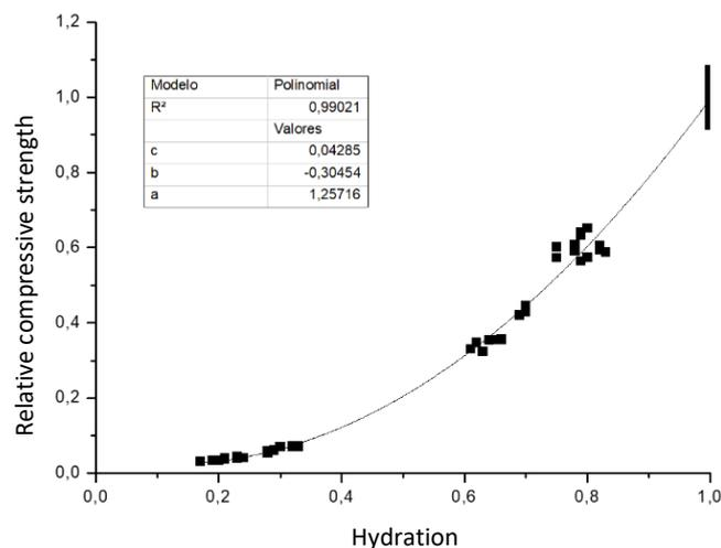
Figure 1. Relation between degree of hydration and relative compressive strength
