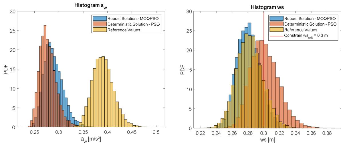
Figure 3. Monte Carlo histograms: at left, weighted acceleration histogram, and at right, working space histogram.
