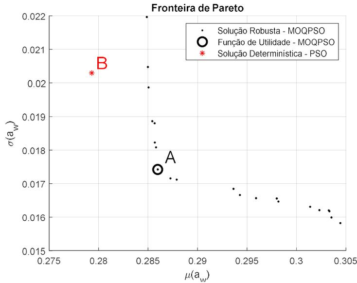
Figure 2. Solution of the RO problem in Pareto Front form (gradient based approximation).
