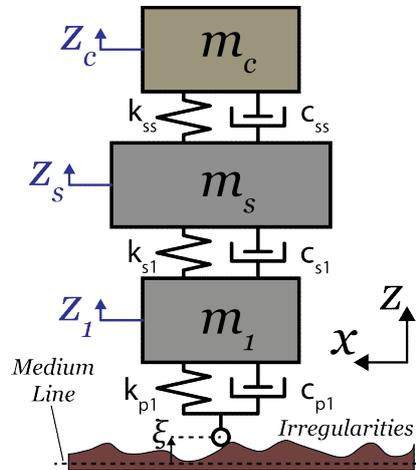
Figure 1. Schematic depiction of the quarter car suspension model used in the simulation.
