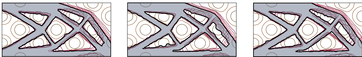
Figure 7. Design domain evolution with d_{sp} = 2\Delta x (left), d_{sp} = 4\Delta x (center) and d_{sp} = 6\Delta x (right)
