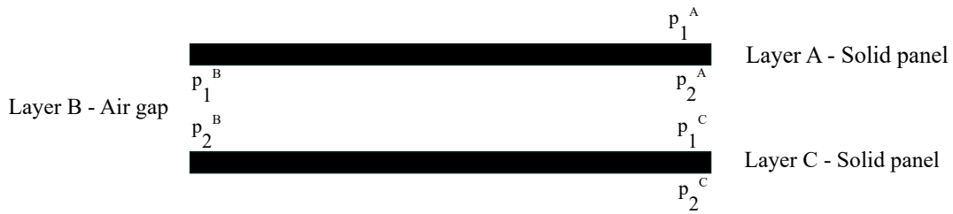
Figure 1. Acoustic pressures ( p ) at different layers of an infinite double panel; A, B, or C superscripts indicate the corresponding layer, and 1 and 2 subscripts indicate acoustic pressure at the upper surface of the layer and bottom surface of the layer, respectively.
