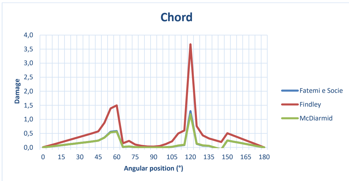
Figure 6. Damage results on the chord area
