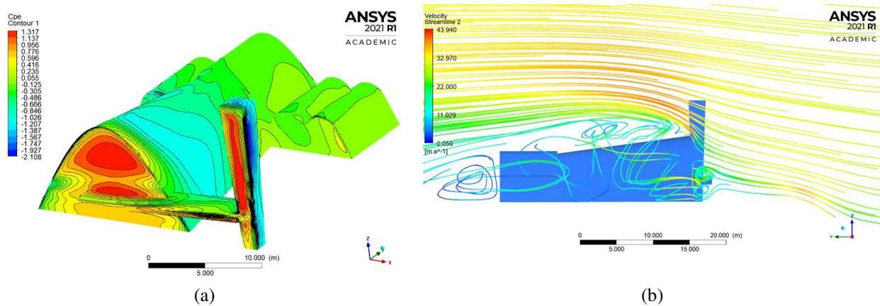
Figure 4: (a) Distribution of pressure coefficients in the building and (b) streamlines in the YZ-plane.
