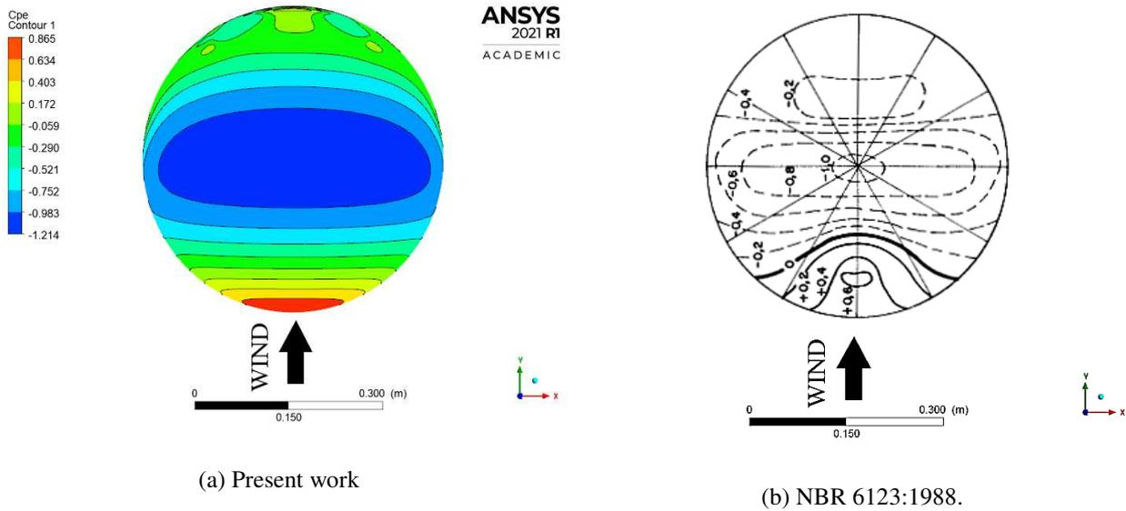
Figure 2. Top view of (a) external pressure coefficients via numerical analysis, and (b) isobaric lines of external pressure coefficients for  $f/d = 1/2$ .
