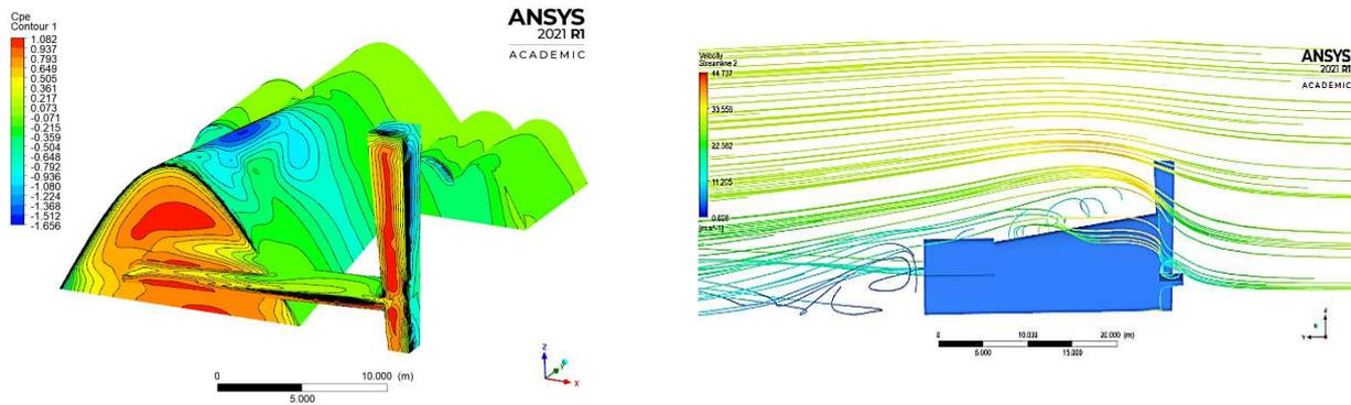
Figure 5: (a) Distribution of pressure coefficients in the building and (b) the streamlines in the building.
