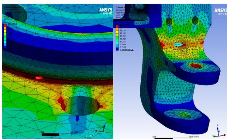
Figure 3. Detected critical points for the steering knuckle. Point “A” on the left, point “B” on the right. Mesh refinement:
