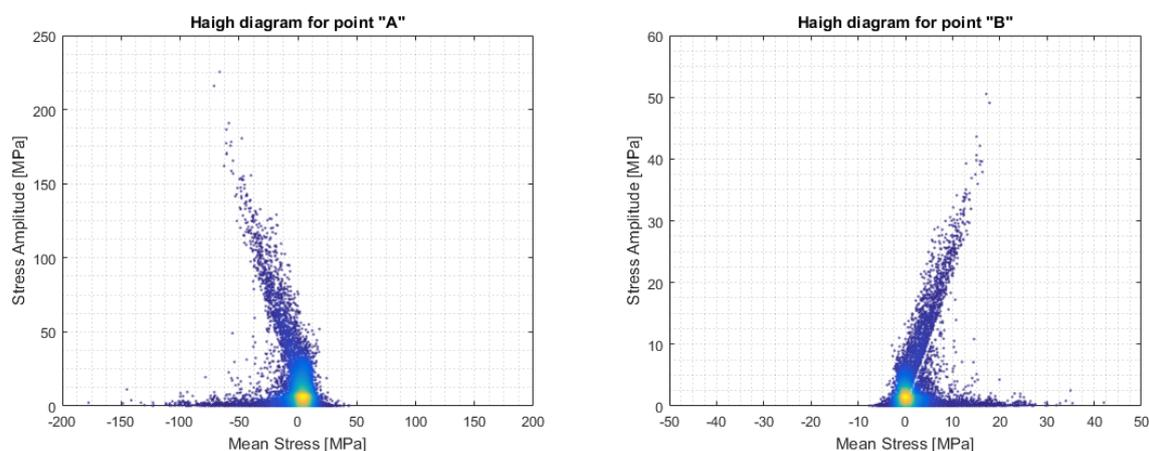
Figure 4. Scatter plots of load cycles on Haigh diagrams for points “A” and “B”, colored by density (brighter colors indicate regions with a higher number of Rainflow cycles).
