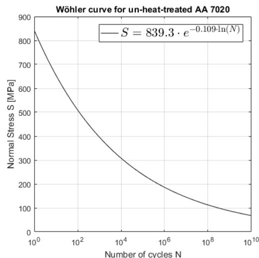
Figure 1. Wöhler curve for AA7020. The exponential characteristic of this S-N curve is representative of aluminum alloys.
