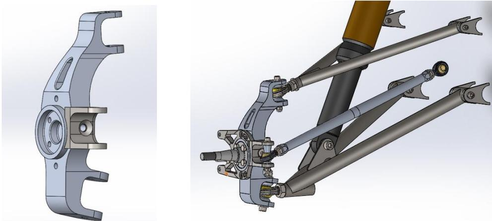
Figure 2. On the left: steering knuckle with support. On the right: frontal-right suspension assembly.
