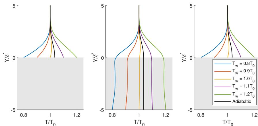
Figure 3. Profiles of flow temperature for various wall temperatures. (Left)  $10\delta_0^*$  upstream from the leading edge of the cavity. (Center) Middle of the cavity. (Right)  $10\delta_0^*$  downstream from the trailing edge of the cavity.
