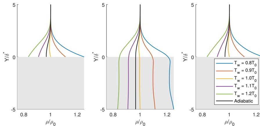
Figure 5. Profiles of flow density for various wall temperatures. (Left)  $10\delta_0^*$  upstream from the leading edge of the cavity. (Center) Middle of the cavity. (Right)  $10\delta_0^*$  downstream from the trailing edge of the cavity.
