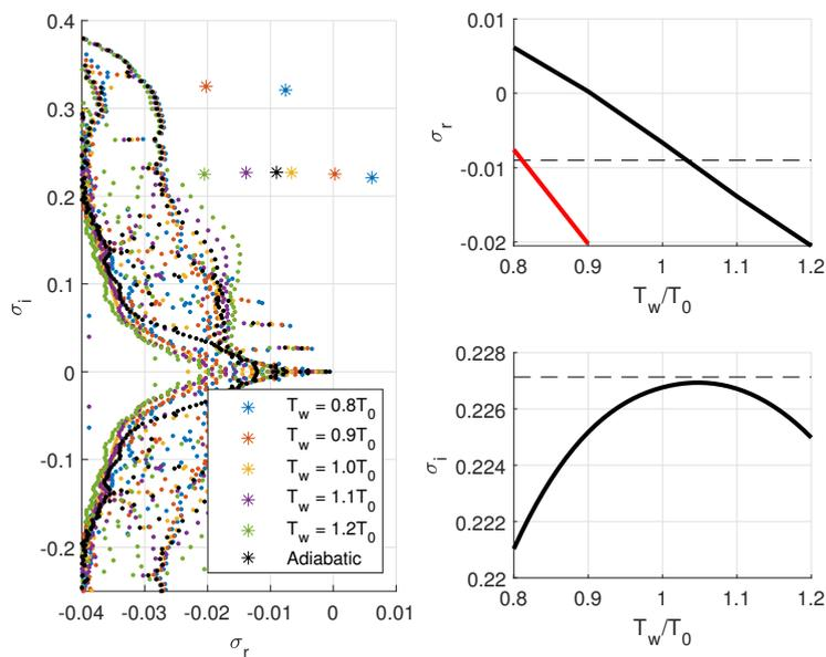
Figure 4. (Left) Global stability eigenvalues for various wall temperatures. (Right) Real part (top) and imaginary part (bottom) of the eigenvalue corresponding to Rossiter mode 1 (black) and mode 2 (red). The dashed line corresponds to the adiabatic case.
