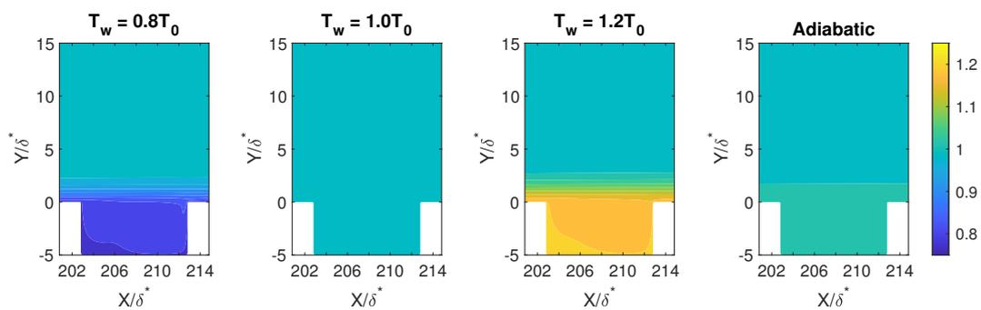
Figure 2. Contours of flow temperature with the wall at 80%, 100% and 120% of the reference temperature.
