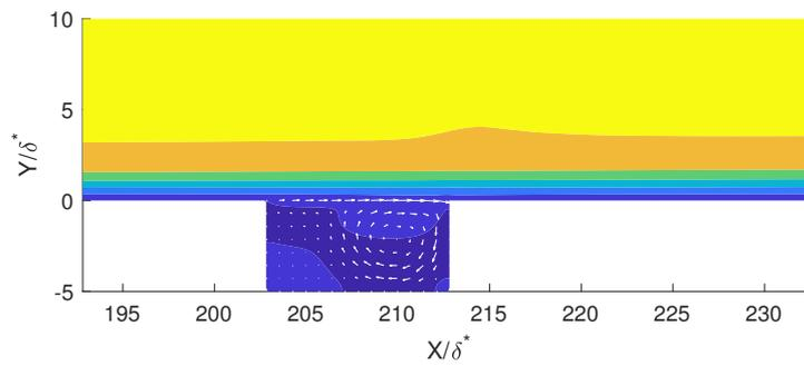
Figure 1. Base flow with the wall at the reference temperature. Contours of stream-wise velocity every 20% of the free-flow velocity.
