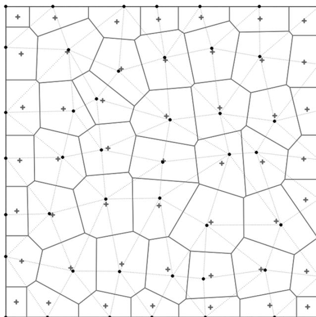
Figure 1. Generating points of *Voronoi* areas (circles) and centroid domain points of *Voronoi* areas (crosses) for an 6x6 nonuniform grid
