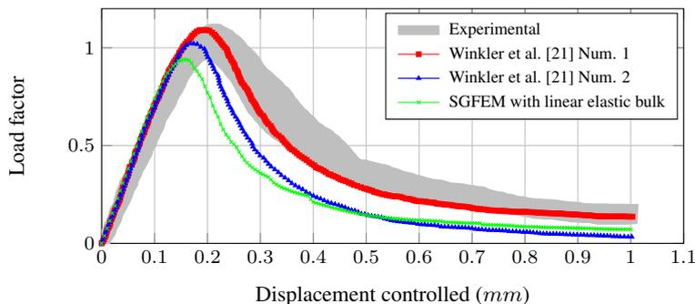
Figure 3. Equilibrium paths obtained for L-shaped panel of Fig. 2. Reference results are taken from Winkler et al. [21].
