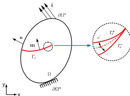
Figure 1. Schematic representation of a solid body in domain  $\Omega$  crossed by a crack  $\Gamma_c$ .
