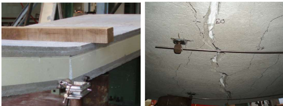
Figure 9. Failure mode of the experimental model – Adapted from Gara et al. [8]
