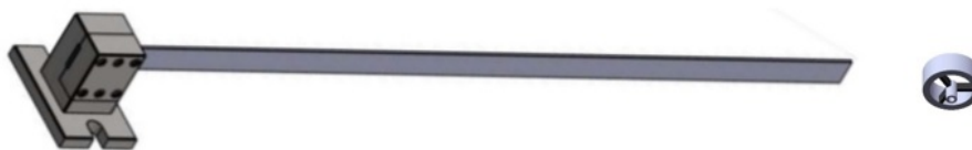
Figure 1. Cantilever Beam + Viscoelastic Dynamic Neutralizer
