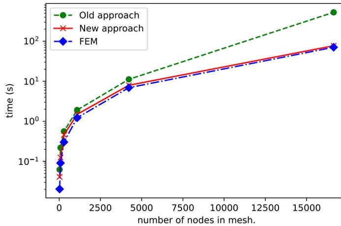
Figure 1. Comparison of processing time of two approaches of the MLGFM.
