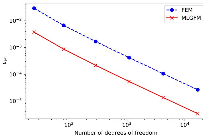
Figure 2. Comparison between MLGFM and FEM on  $L_2$  error norm for domain source example.
