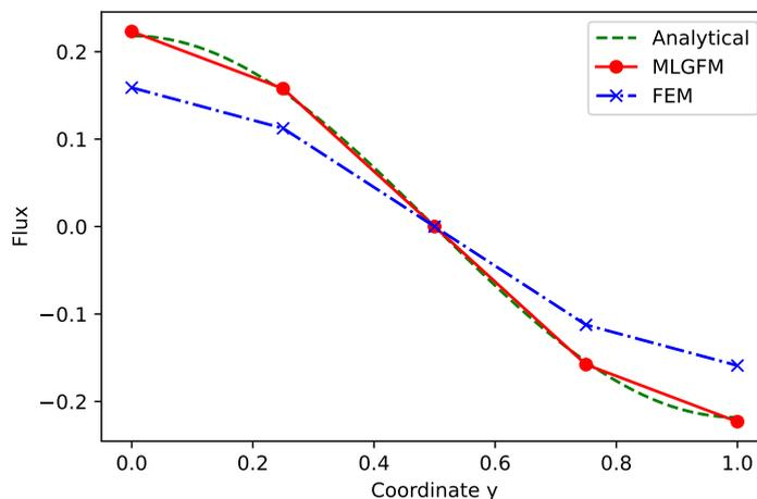
Figure 3. Comparison between MLGFM and FEM flux results in  $x$ -direction for domain source example.
