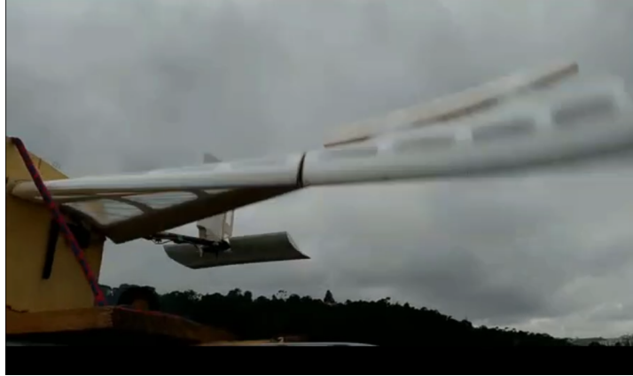
Figure 2. Example of structural response to torsional displacement of a wing.
